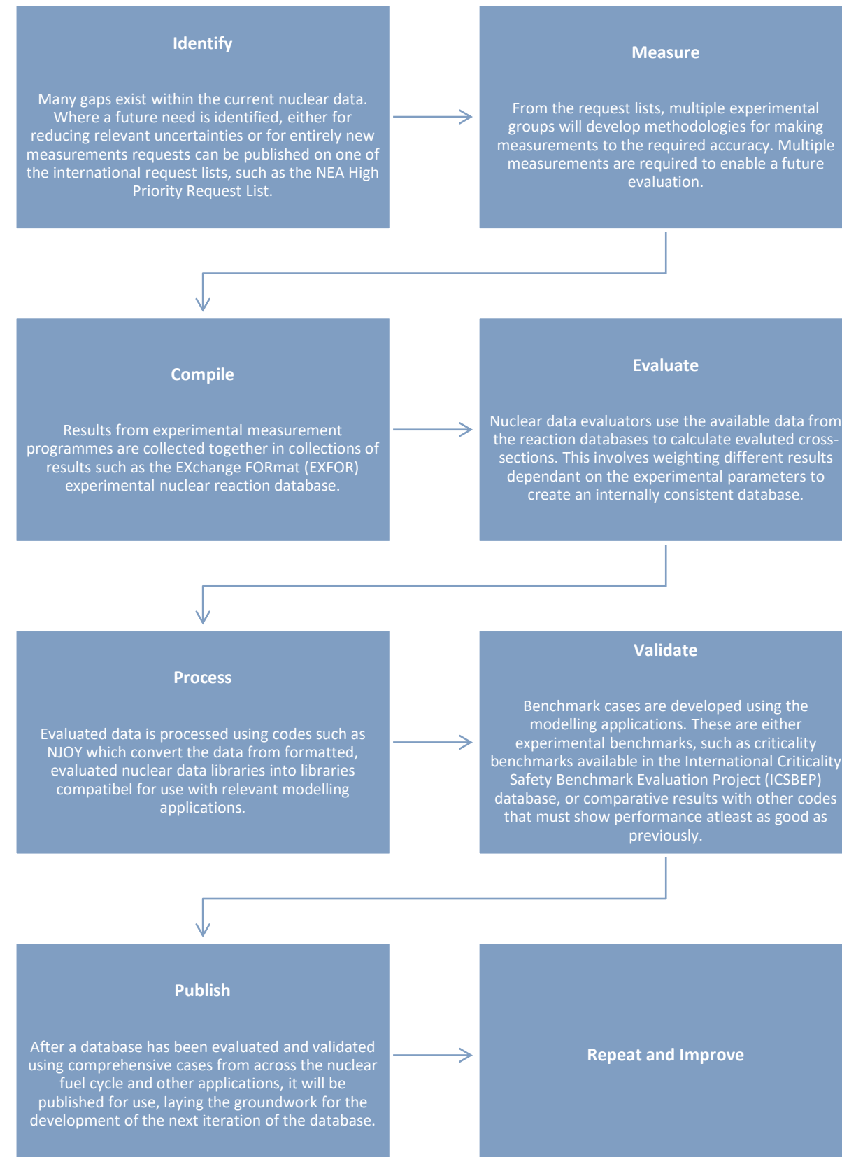
Figure 1: Outline of a simplified nuclear data lifecycle highlighting the key steps in the process.
