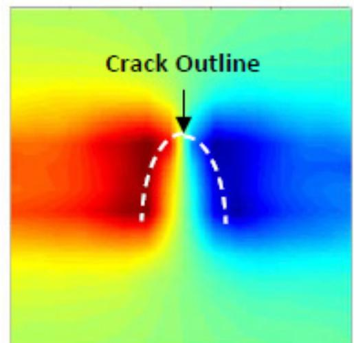
*Magnetic field distribution of NNUMAN weld sample with crack defect*
