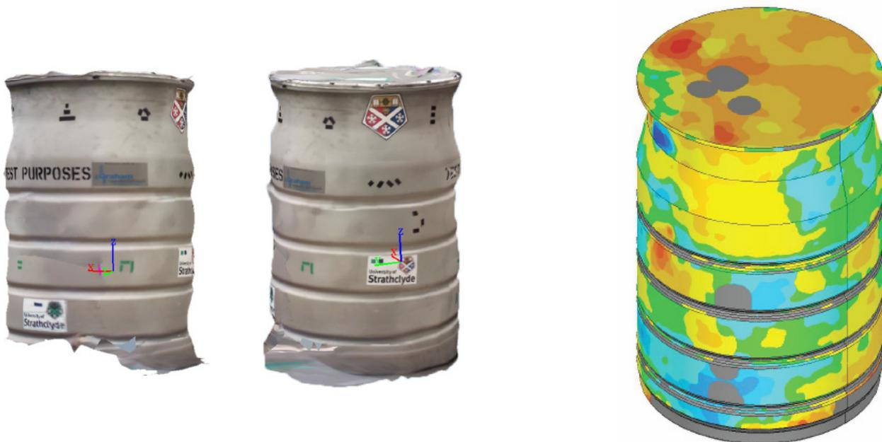
**Above Left:** 3D surface-meshed model of ILW container. **Above Right:** Comparison of the photogrammetry to actual dimension measurements
