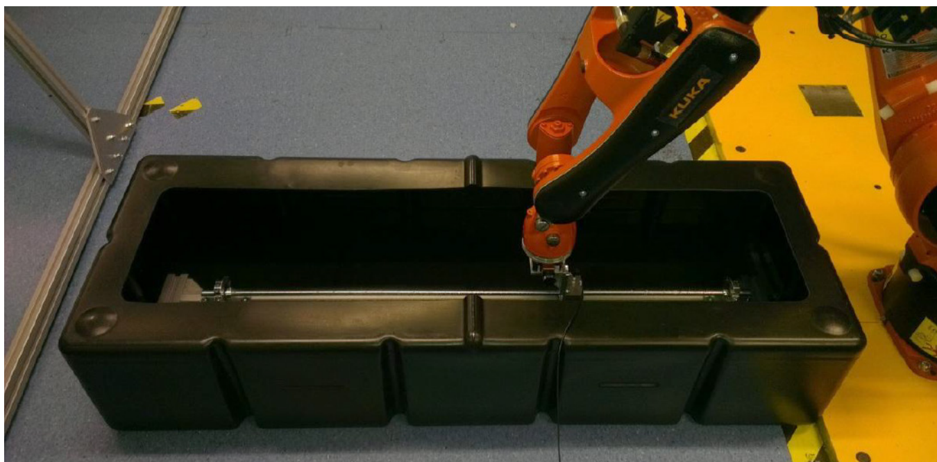
Above: The eddy current probe connected to a fixed arm robot scanning a dummy AGR fuel pin submerged in water. Below: Eddy current response for a complete helical scan of the fuel pin with the fifteen defects.
