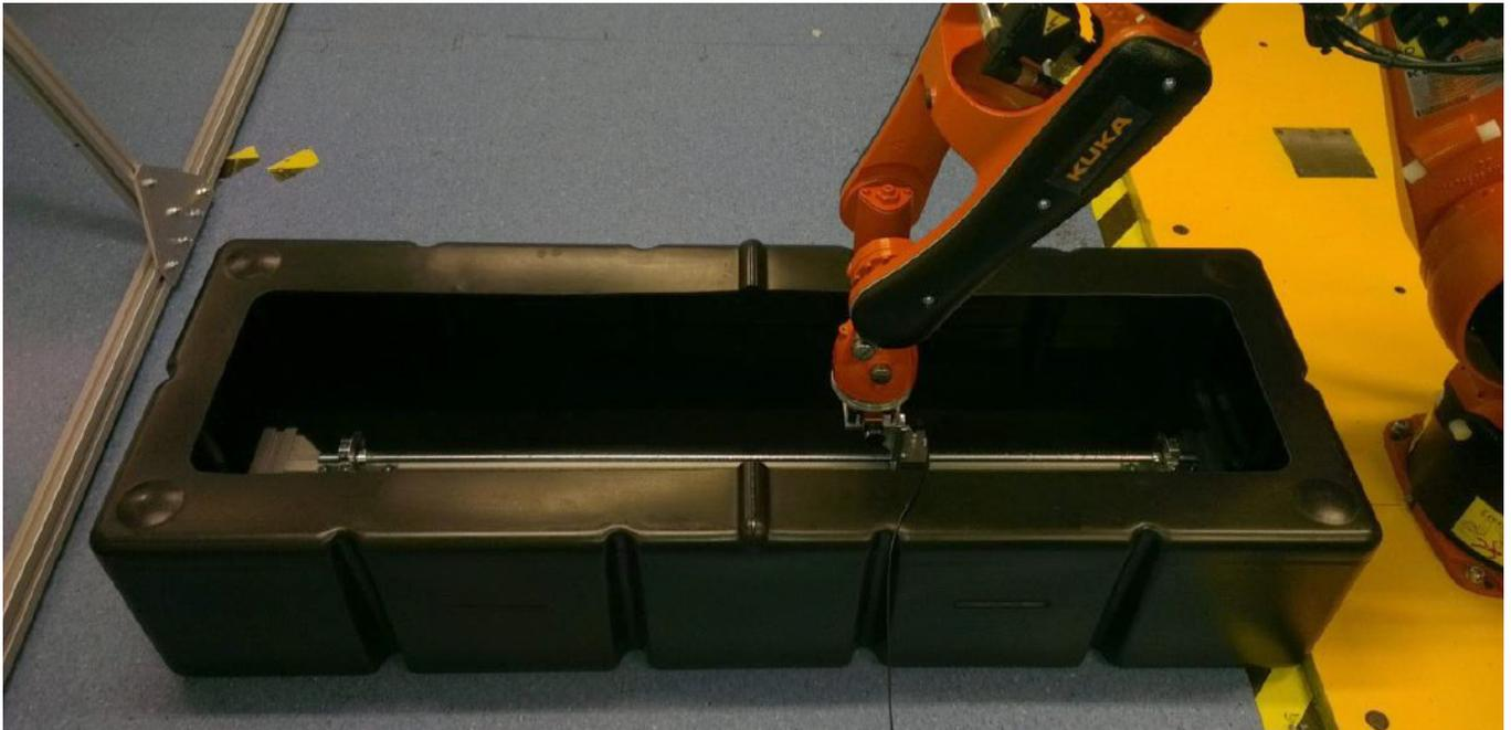
**Above:** The eddy current probe connected to a fixed arm robot scanning a dummy AGR fuel pin submerged in water. Below: Eddy current response for a complete helical scan of the fuel pin with the fifteen defects.
