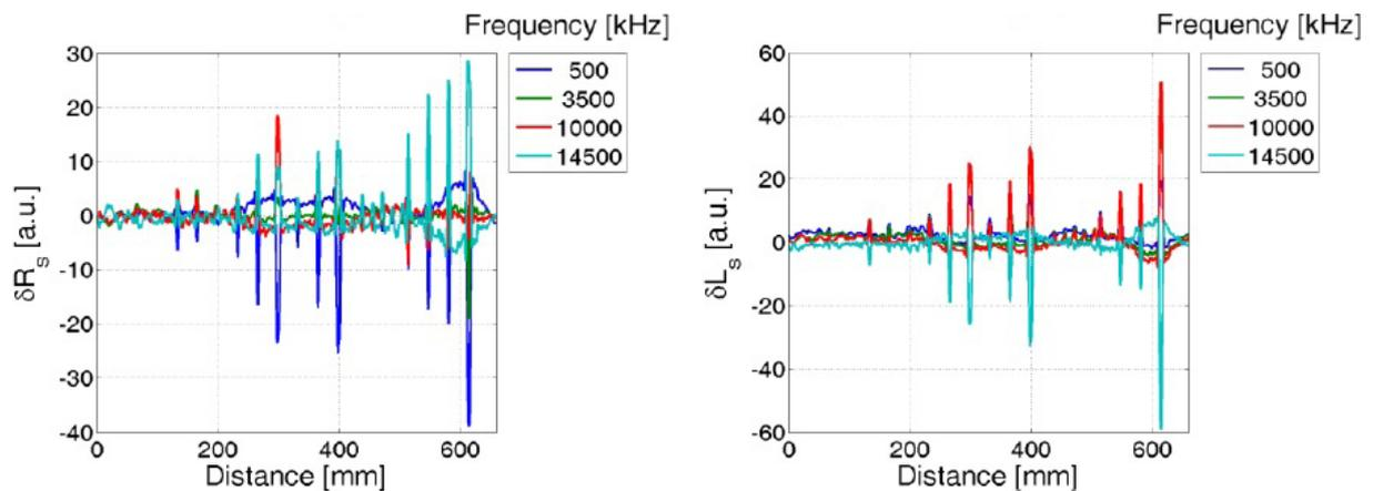
Grooves (ASGs) on the fuel pin. Using the SFEC approach, signals are collected at multiple frequencies and it is recommended that further work is performed on signal processing and defect recognition algorithms as the signals caused by changing stand-off and defects may have different spectral effects.
