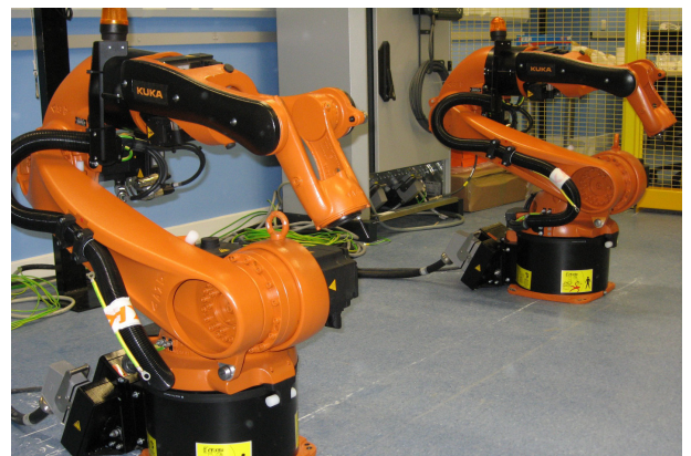
FIRST Lab: 6 axis kuka robotic arms
