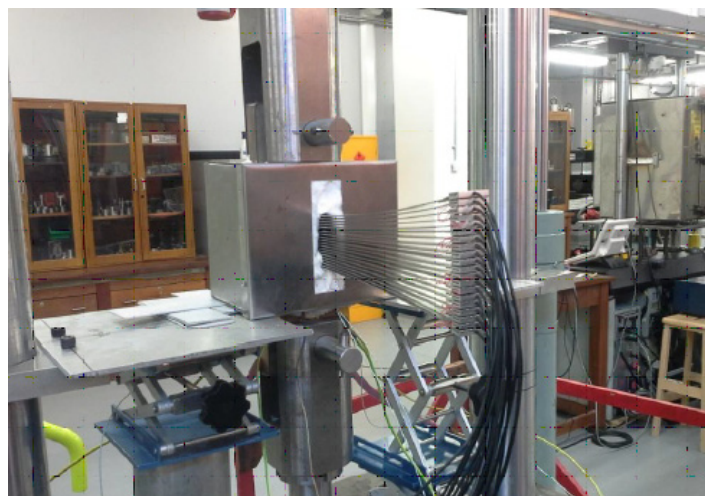
Above: Wave guides exiting a furnace containing the sample
